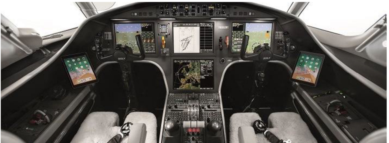
Figure 9: Render showing deployed iPad locations on F900EX EASy series (F2000EX EASy series similar)
