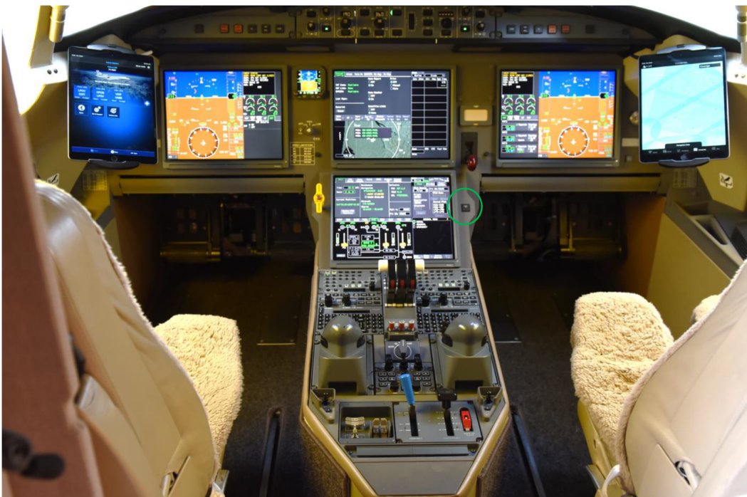
Figure 7: Deployed Cockpit Mounts on 7X with power off switch (circled in green)
