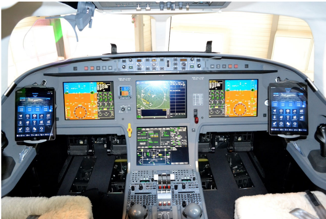
Figure 6: deployed Cockpit mounts on 8X with power off switch between co-pilot console and RH cockpit sidewall (not shown)
