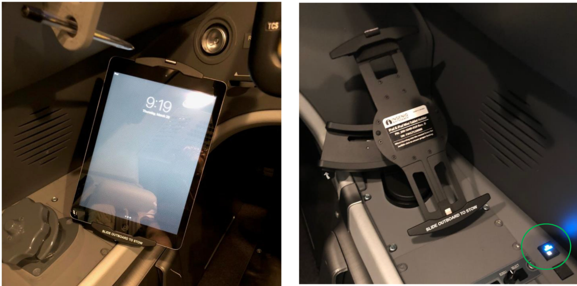
Figure 10: Pilot side cockpit mount deployed (left); copilot side cockpit mount stowed with charging switch circled in green (right) - F2000EX EASy and F900EX EASy series
