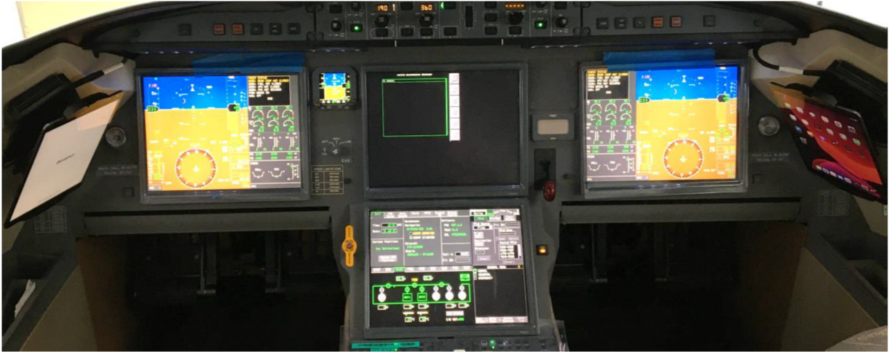
Figure 8: Stowed Cockpit iPad Mounts on 7X
